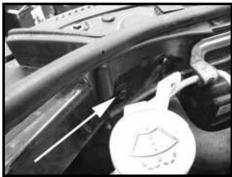
Step 12 Remove the bolt on the core support. This will be reused in the next step.
