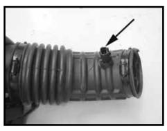
Step 6 Turn the IAT sensor counterclockwise and remove it from the factory intake tube. Remove the O-ring from the sensor.
