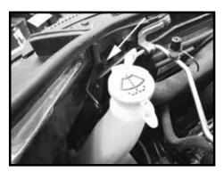
Step 13 Install the bracket with bolt removed in the previous step. The large hole is used to mount the bracket to the core support.
