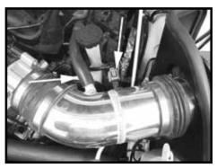
Step 17 Trim the factory breather hose to length and install onto the nipple on the intake tube. Reconnect the IAT sensor connector.
