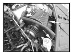
Step 14 Install the heat shield assembly in the vehicle. Align the grommets onto the pins located on the inner fender as well making sure the bracket is on the flex coupler side of the heat shield.
