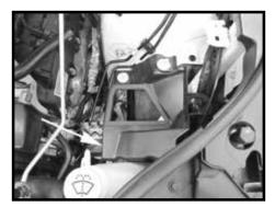
Step 5 Remove the lower air box tray out of the vehicle.
