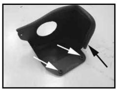
Step 9 Install the rubber bulb seal, this may require trimming to the correct length. Install the grommets removed from Step 8.
