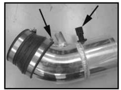
Step 7 Install the supplied grommet into the intake tube then install the IAT sensor into the grommet. Install the reducer coupler onto the end of the tube and fasten it securely, leave the other clamp loose at this time.
