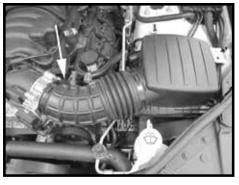
Step 4 Loosen the clamp at the throttle. Remove the factory air intake system from the vehicle.
