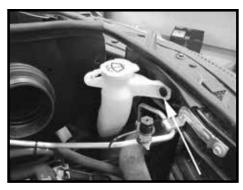
Step 15 Reinstall the panel clip and center pin that was removed in Step 11.
