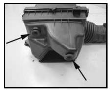
Step 8 Remove the factory grommet from the air box. This will be reused on the next step.
