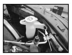
Step 11 Remove the center pin using a screwdriver to help remove the center pin. Once the center pin is removed, remove the panel clip from the vehicle. This will be reinstalled in a later step.
