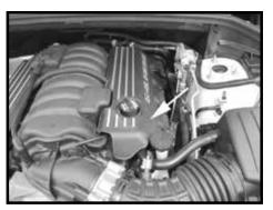
Step 2 Remove the engine cover.
